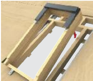
Install roof window frame
