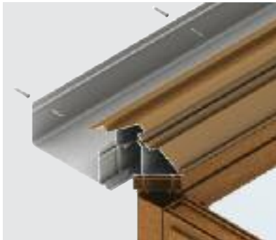
Fix box gutter to existing wall
