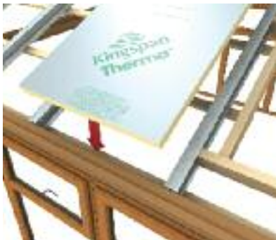
Install external insulation
